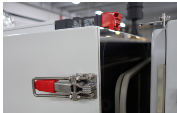
MAGNETIC DOOR LOCK AND MANUAL LATCHES
